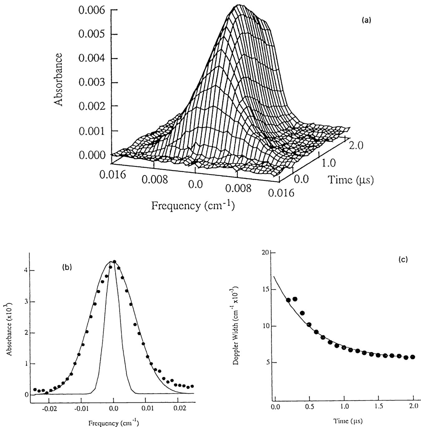
Figure 4. Time-resolved sub-Doppler spectroscopy of  $\text{CO}(v=0, R19)$  from  $\text{H} + \text{OCS} \rightarrow \text{CO} + \text{SH}$ ; (a) absorbance as a function of frequency and time, (b) lineshape, Gaussian fit, and 298 K reference lineshape at 500 ns following the photolysis pulse, (c) Doppler width versus time extrapolates to  $0.0168 \text{ cm}^{-1}$  at  $t=0$ .
