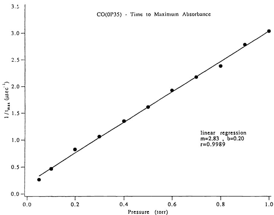
Figure 2. The time to maximum signal amplitude for CO( $v=0, J=35$ ) from  $H + OCS \rightarrow CO + SH$  shows the pressure dependence predicted by the model.
