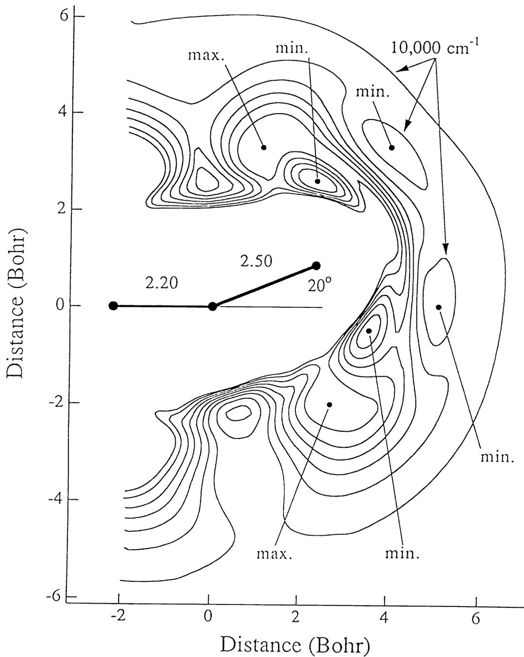
Figure 5. H atom energy contours for H+CO<sub>2</sub> at the cis saddle point geometry. Contours are separated by 2500 cm<sup>-1</sup>; the highest is at 25,000 cm<sup>-1</sup>.
