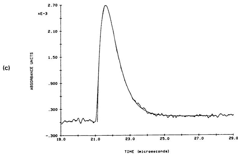
Figure 1. CO( $v=0$ ) transient absorption signals from  $H + OCS \rightarrow CO + SH$ ; (a) P(10), (b) R(20), (c) P(35).
